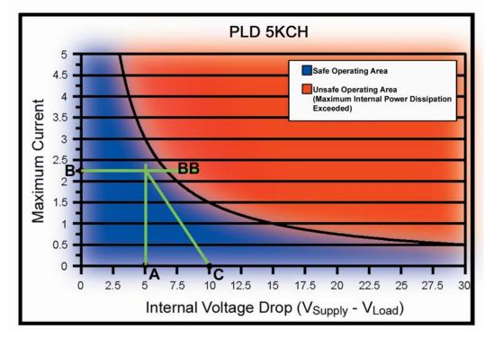
\*Derate maximum power dissipation 1.3 Watts / °C for chassis temperatures above 55 °C
