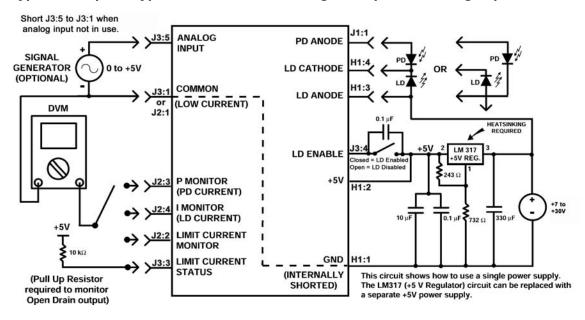
\*Note: When configuring the PLD10K-CH and PLD5K-CH for High Compliance operation, the jumper must be cut on Terminal Block H1 between pins 2 and 3. This allows the addition of a separate power supply to the laser diode anode (H1, Pin 3). See the diagram below for the location of the jumper.
